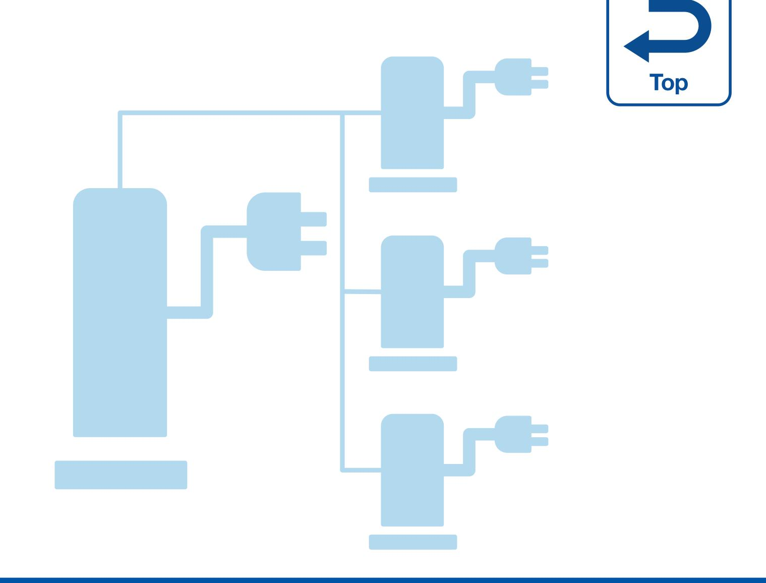
■ By integrating a main unit that has communications, verification, billing, and charging functions with sub-units that are dedicated to charging, new and additional installation costs are reduced when installing multiple charging stands.
