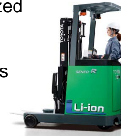
Electric lift truck with lithium-ion battery
