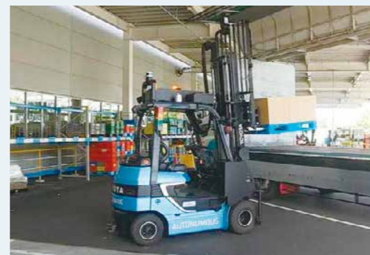
Feasibility test of an automated guided forklift
