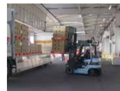
Automated truck loading/ unloading by AGF
