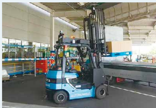
Feasibility test of an automated guided forklift
